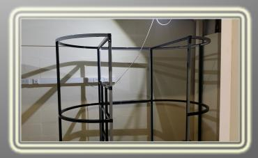
16. Beam C4 and the remaining beam which the curtain goes onto can then be fitted. These have to be put into the blocks simultaneously. Connect the two beams into one side of the booth first but don't twist into position. The beams are then fitted into the opposite side of the doorway making a full connection, they can then be twisted into place.
